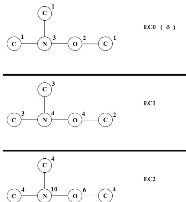
Fig. 4. Example of calculation of the Morgan extended connectivity (EC) of first and second orders. The zero-order EC0 is the vertex degree  $\delta$ .
