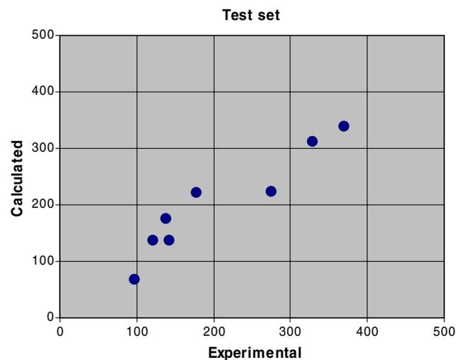
Fig. 2. Correlation between experimental and calculated Young's modulus (in GPa) values for the test set.
